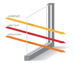
Without Window Film **One-third** of a building's cooling load is from solar heat gain through windows
